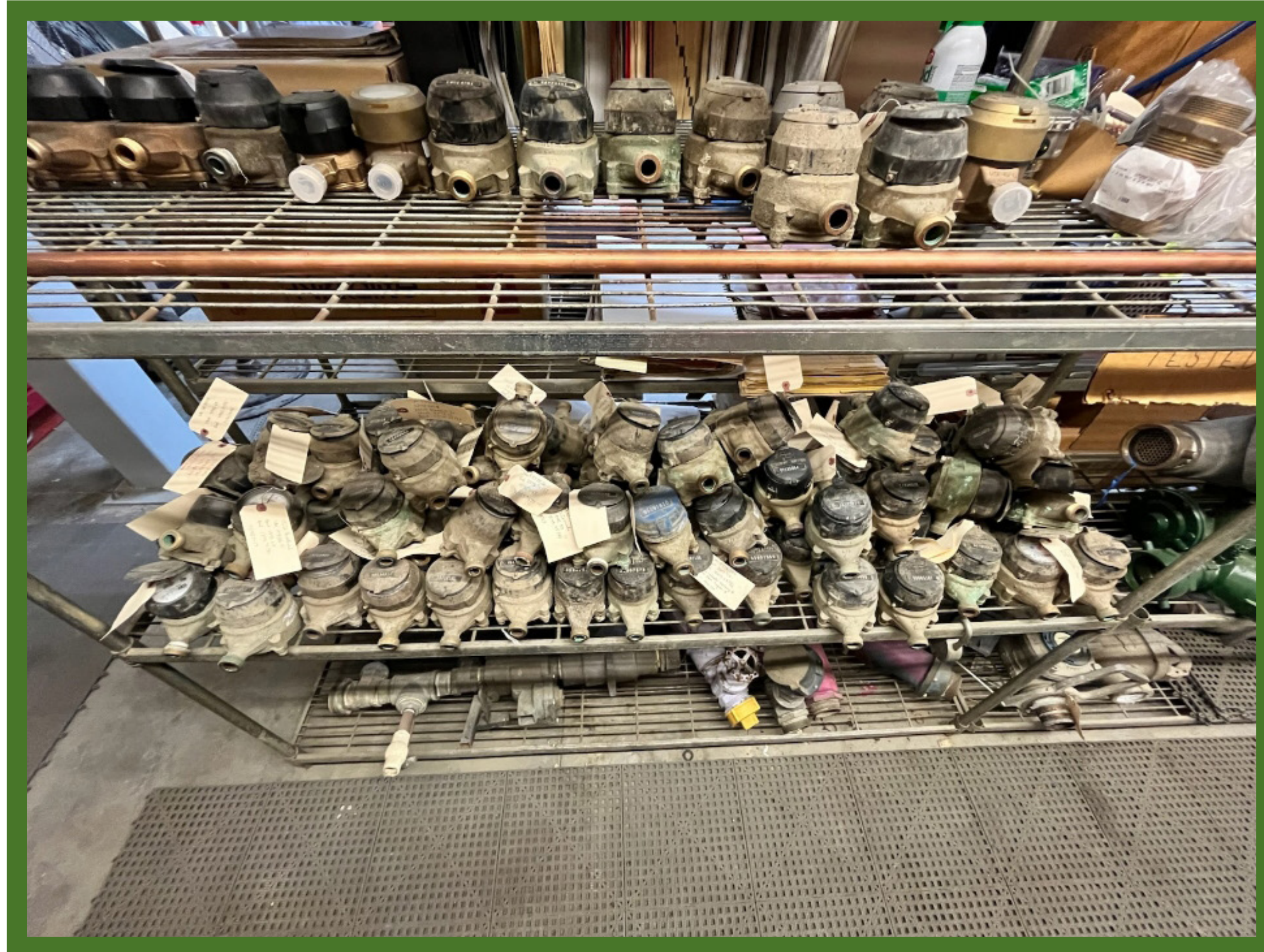
Top: New meters Bottom: Old, non-registering meters
